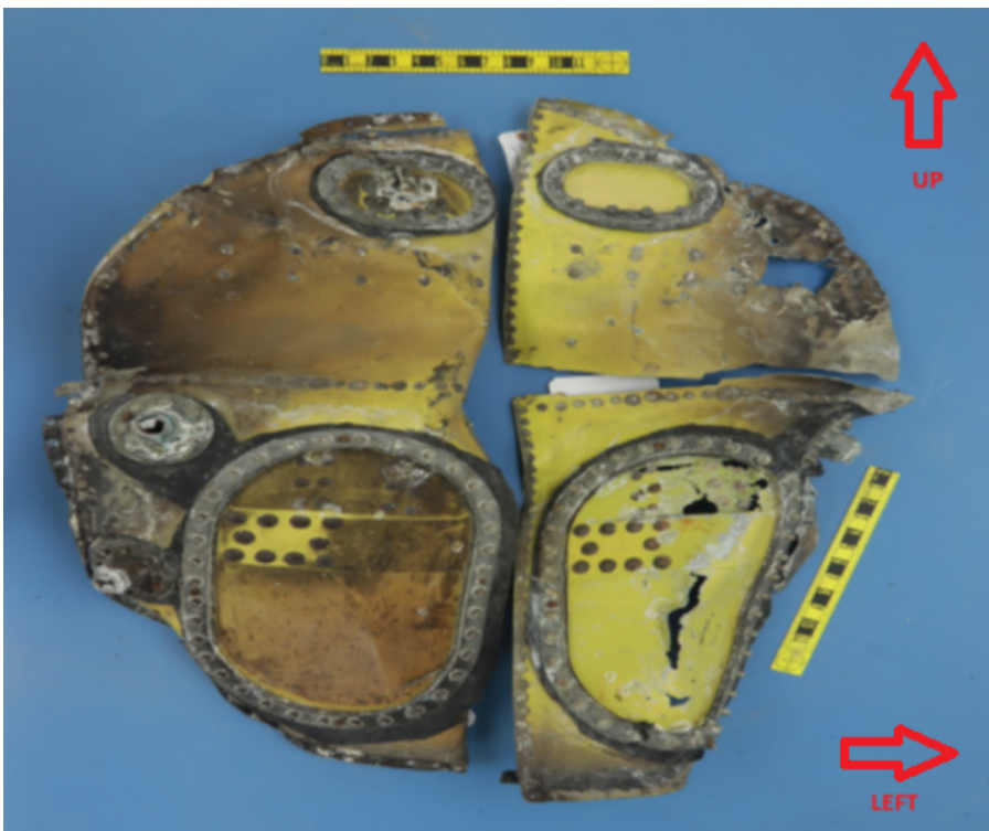
Figure 6 – Fuselage Fuel Tank Bay Aft Bulkhead (Forward Facing Side)
