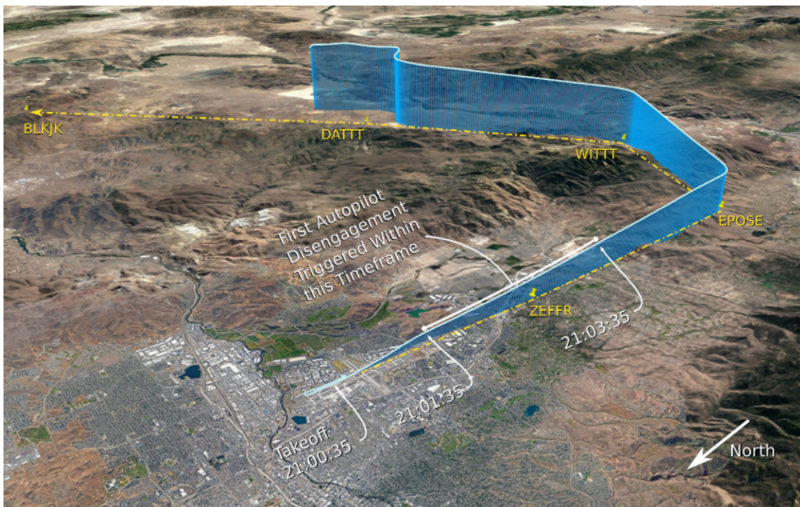
Figure 3: CAWS data map overlay showing the takeoff event and first autopilot disconnect.
